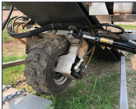
Hydraulic driven and steerable drive wheel
