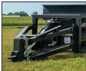
Remote controlled belt and tow hitch.
