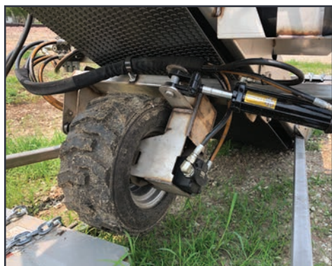
Hydraulic driven and steerable drive wheel
